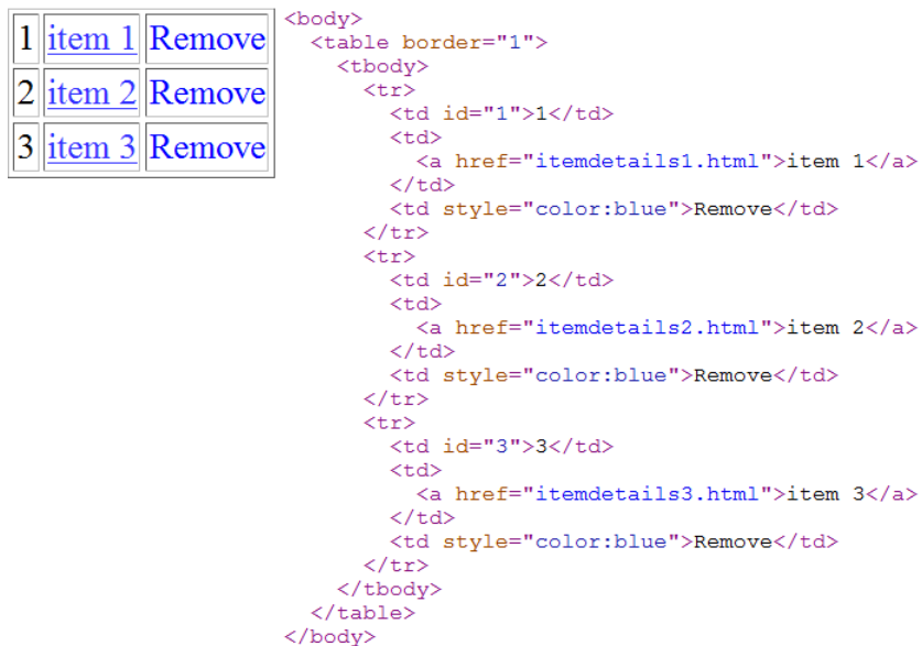
Figure 2: A page containing a table (left) and the body of the corresponding HTML document (right)
